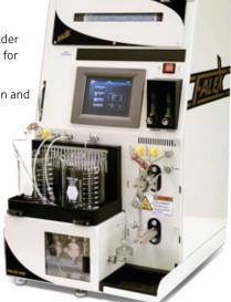
Falex 430 Ellipsometer for Rating Deposits on ASTM D3241 Heater Tubes
