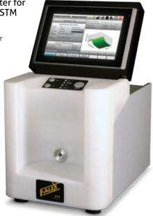
The Falex ETR offers a simple one button operation for use with all aluminum heater tubes and all ASTM D3241 instruments.
