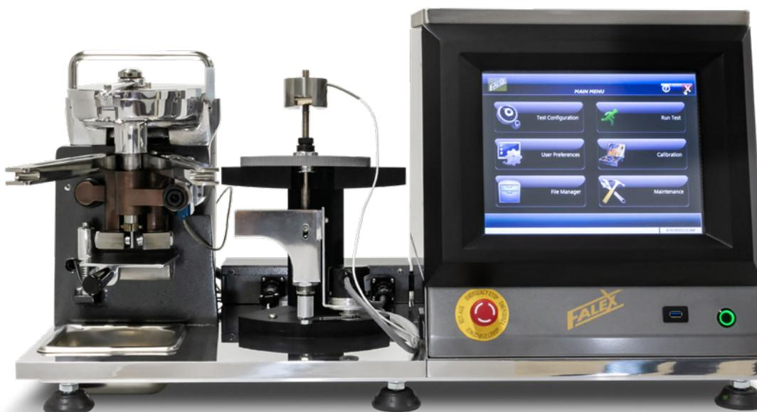
The versatile, Falex Pin and Vee Block Machine is used to evaluate wear, friction, and extreme pressure properties of lubricants, coatings, and materials in a multitude of applications. The latest model features an integrated touchscreen computer system for easy operation, calibration, data acquisition, and test reports. Custom test pieces are available from other materials to better match field conditions.
